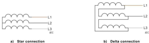
Figure 5 – Three-phase three-wire system
